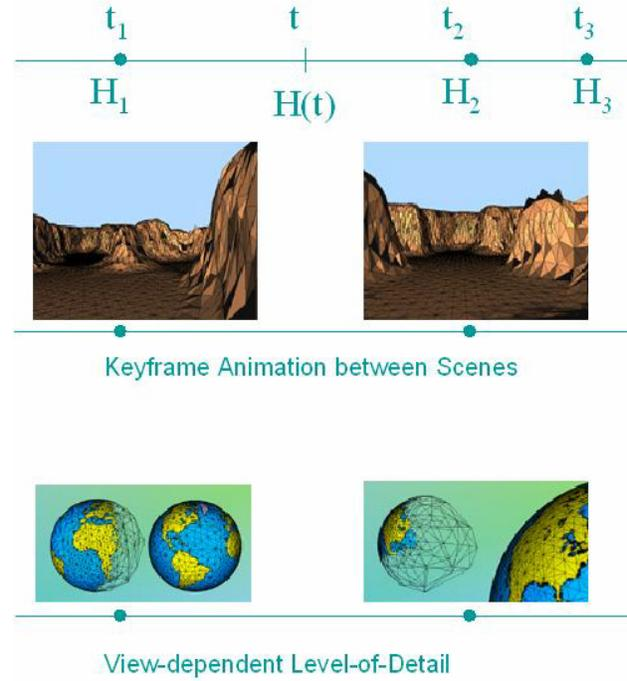
Figure 5: Interpolation between view-dependent keyframe representations  $H(t_1)$  and  $H(t_2)$  at times  $t_1$  resp.  $t_2$  of an animated scene. Since the view-dependence computation has been performed on the keyframe representations, the interpolated representation  $H(t)$  can be rendered directly. This approach avoids the view-dependence computations at every frame.
