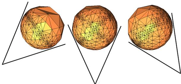
Figure 1: Left and right image show view-dependent representations of a sphere depending on the indicated camera position. The middle image shows the sphere at an intermediate time. Its rendered mesh has been obtained by interpolating the two view-dependent meshes of the adjacent keyframes, thereby avoiding a new view-dependence computation.
