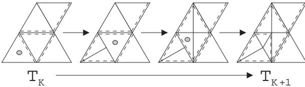
Figure 3: A single step of the Rivara/Bänsch bisection method with refinement edges and marked triangles.
